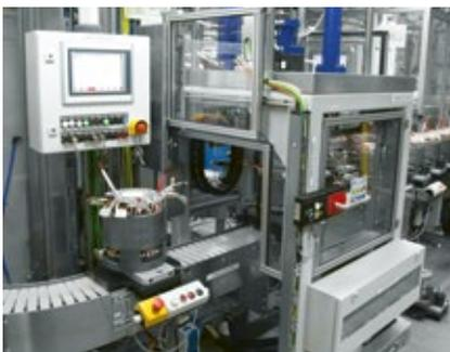
Final process of slot wedges compacting.
