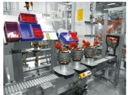
Winding heads phases insulation process.
