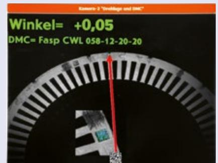
Geometric test by 2D Video camera.
