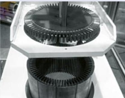
Geometrical test by mechanical calibre.
