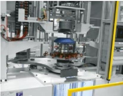
Coil inserting process by high efficiency insertion technology.
