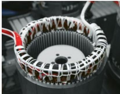
Winding head lacing machine on leads stator side.
