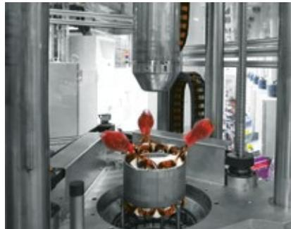
Winding heads Expanding process.
