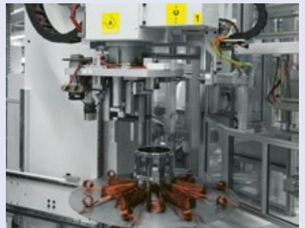
Coil winding and wedge making process.
