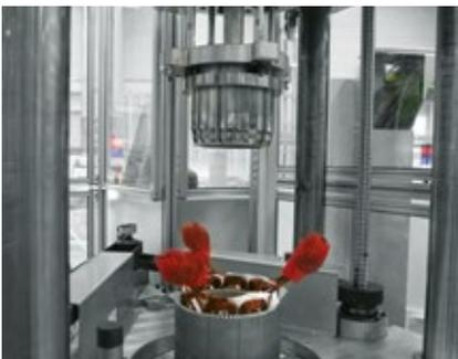
Intermediate and final winding heads forming process.
