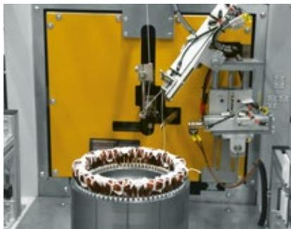
Winding head lacing machine on opposite leads stator side.
