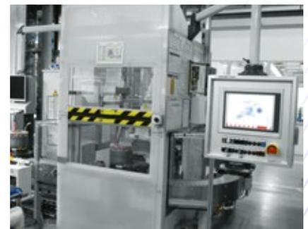
End coil winding process with in line electrical test.
