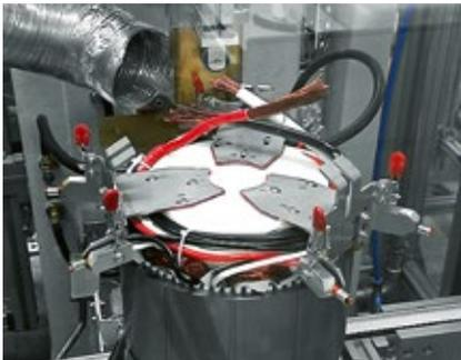
Automatic winding leads connection process.
