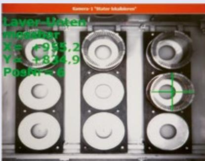
Boxes for stators unload with 2D vision by camera.
