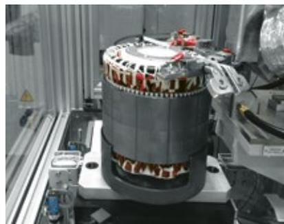
Automatic winding leads connection process.
