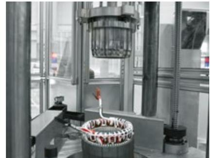
Intermediate and final winding heads forming process.
